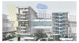
Sustainable design features in Centennial Village include stilted infrastructure to withstand projected flooding during Category 5 hurricane high tides, bioswales for stormwater management, active chilled beam HVAC design, self-shading exterior elements to conserve energy, and direct air systems with enhanced filtration and recovery. Check out the virtual tour <u>HERE</u>!
