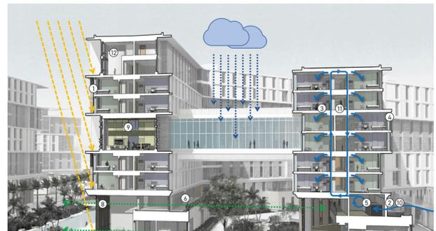
Sustainable design features in Centennial Village include stilted infrastructure to withstand projected flooding during Category 5 hurricane high tides, bioswales for stormwater management, active chilled beam HVAC design, self-shading exterior elements to conserve energy, and direct air systems with enhanced filtration and recovery. Check out the virtual tour [HERE!](#)
